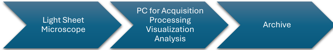
Figure 2: Example Basic Configuration Single Computer Workflow for Light Sheet Microscopy Description: The central panel represents the PC for all tasks including acquisition, stitching, compression, deconvolution, visualization and analysis. Arrows indicate data flow.
