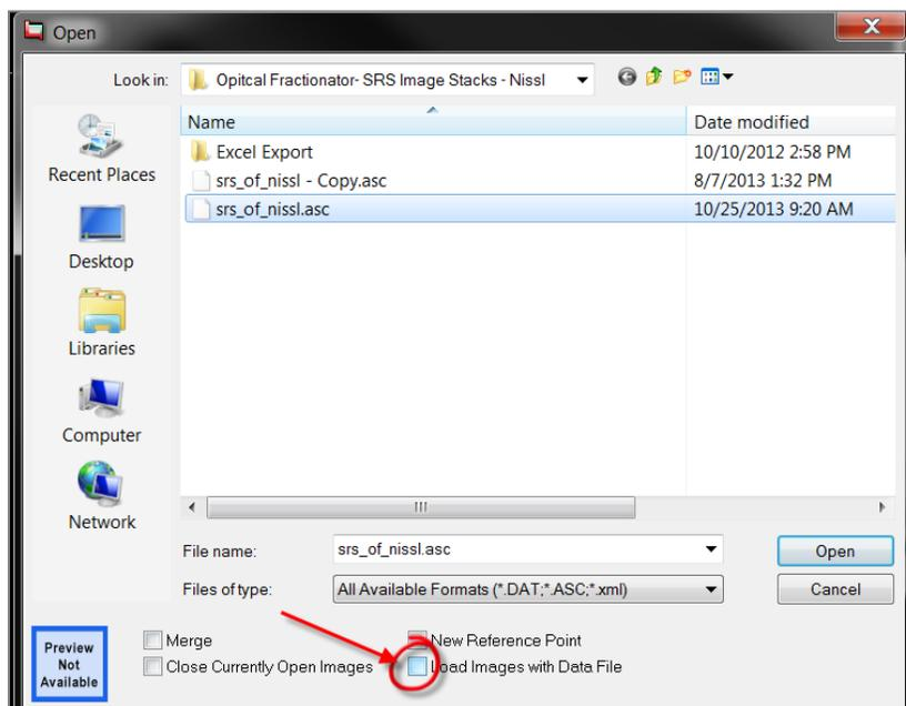
3. The *Open* dialog box is displayed. Select the desired data file, uncheck **Load Image with Data File** (recommended for faster performance), and click **Open**.
